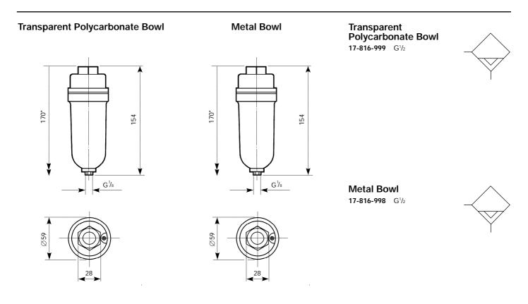
\*Minimum clearance required to remove bowl from body.
